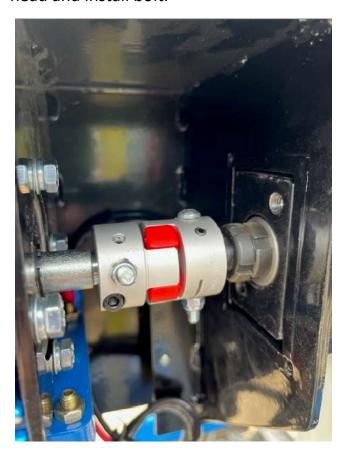
6. Evenly screw in set screws and tighten with lock nuts.
