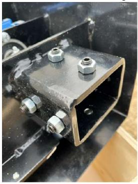
5. Align the holes on the shaft with the old crank handle. Once aligned, slide on new power head and install bolt.
