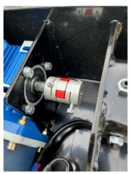
3. Remove bolt on Lovejoy connection of new electric motor.
